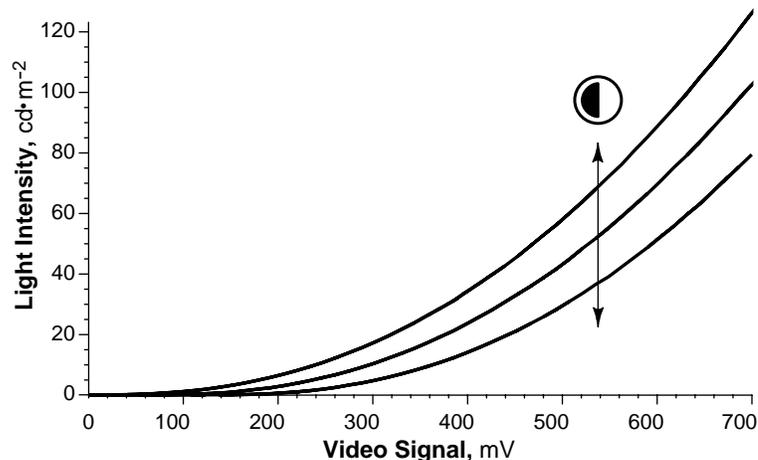
This graph indicates a video signal having a voltage from zero to 700 mV. In a typical eight-bit digital-to-analog converter on a framebuffer card, black is at code zero, and white is at code 255.
