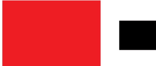
Image sensor size comparison: 8.0 megapixel Digital Rebel XT (Red) vs. 8.0 megapixel compact digital camera (Black)
